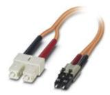
Assembled FO cable, zip cord cable, multi-mode fiberglass 62.5/125 µm, OM1, connector: SC duplex/LC duplex, degree of protection: IP20, for installation in cable ducts or control cabinets
