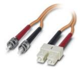
Assembled FO cable, zip cord cable, multi-mode fiberglass  $62.5/125 \,\mu m$ , OM1, connector: SC duplex/B-FOC (ST), degree of protection: IP20, for installation in cable ducts or control cabinets
