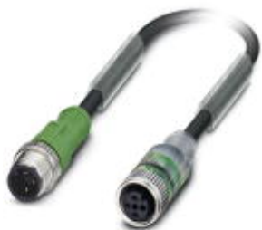
Sensor/actuator cable, 3-position, Variable cable type, Plug straight M12, A-coded, on Socket straight M12, A-coded, with 2 LEDs, cable length: Free input (0.2 ... 40.0 m)
