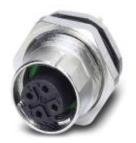
Bus system flush-type socket, Ethernet, 4-pos., M12 SPEEDCON, D-coded, rear/screw mounting with Pg9 thread, with straight solder connection, design with 12 mm long solder pins
