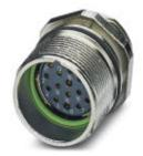
Device connector for front wall, straight, shielded: yes, SPEEDCON locking, M23, No. of pos.: 16+2+PE, type of contact: Socket, Crimp connection, Axial seal, Central fastening Pg13,5
