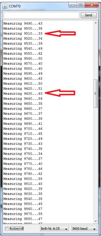
The larger the number the higher the transmission power. For example, 96.3MHz is a higher number than the others (<u>FYI</u>, its <u>Univision 96.3 FM</u> (http://adafru.it/dBs)!) whereas 95.1 MHz is nice as low, that's not used for any transmission. Try to find a number that's also not surrounded by high numbers, since it can get 'drowned out' by the nearby
