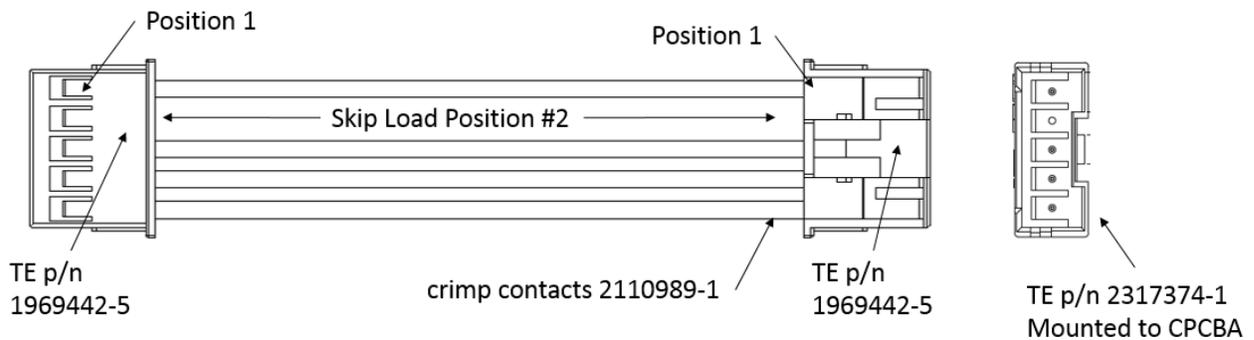
Figure 11. EMC Cable Assembly, TE p/n 2318044-1
