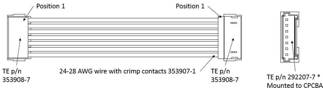
Figure 9. LCC Cable Assembly, TE p/n 2318043-1
