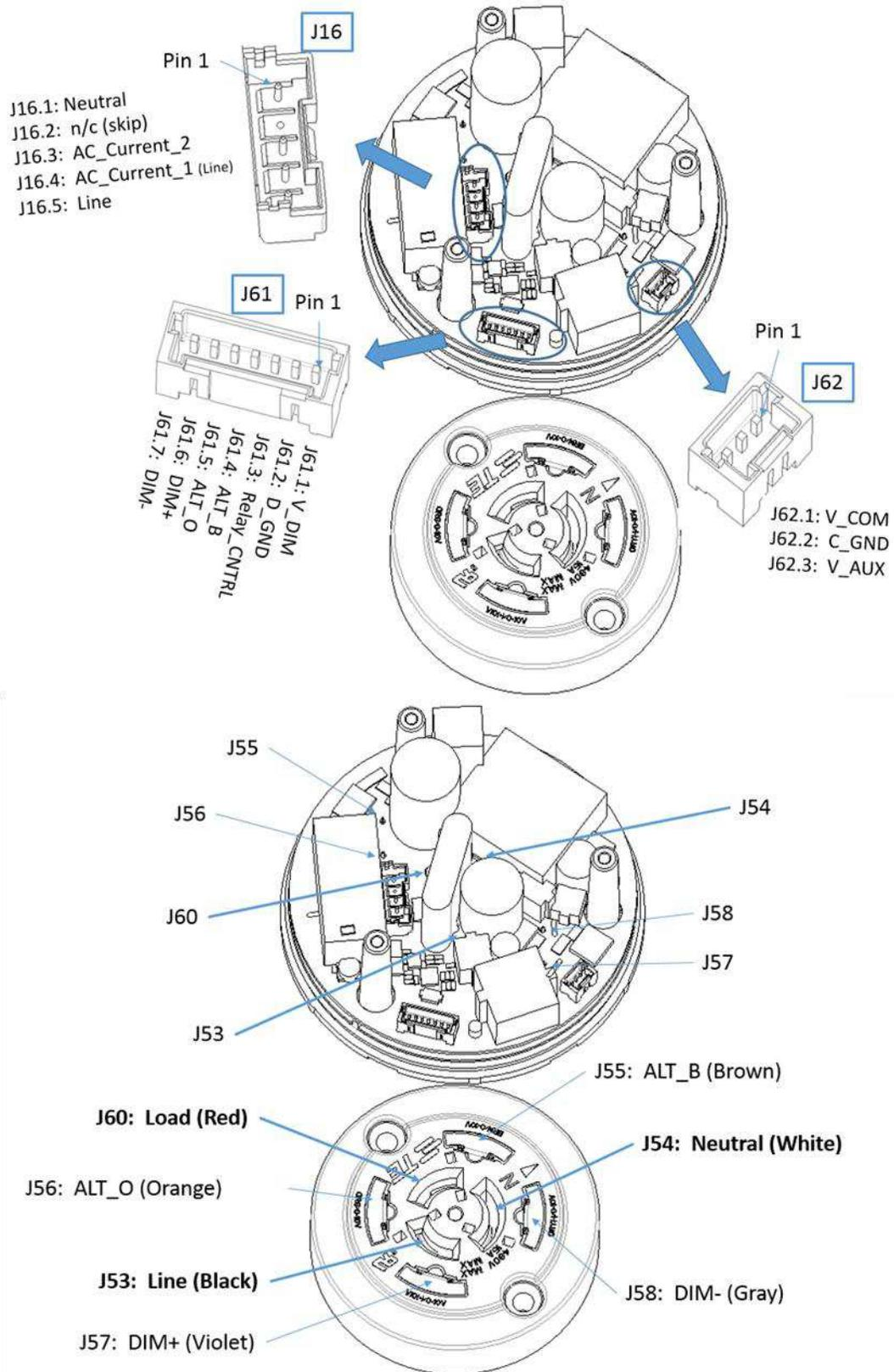
Figure 3. Enhanced Base Pinout / Contact Arrangement
