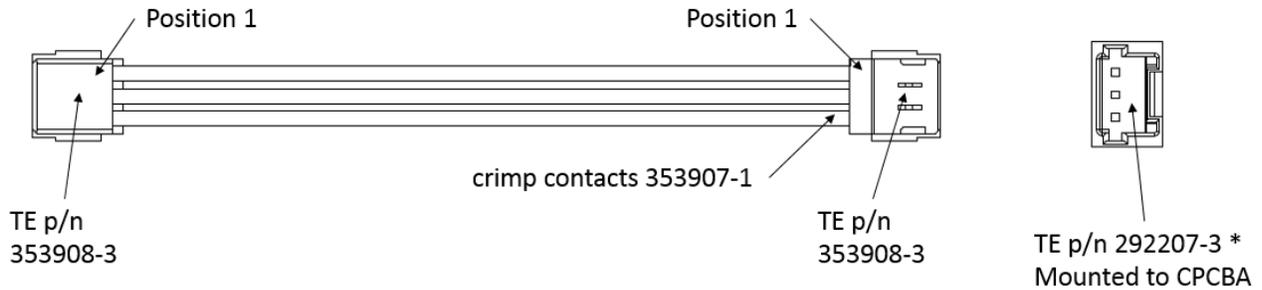
Figure 10. MPC Cable Assembly, TE p/n 2318043-2
