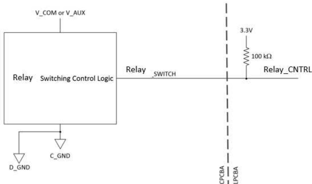
Figure 5, Relay Switching without Energy Metering (Example)
