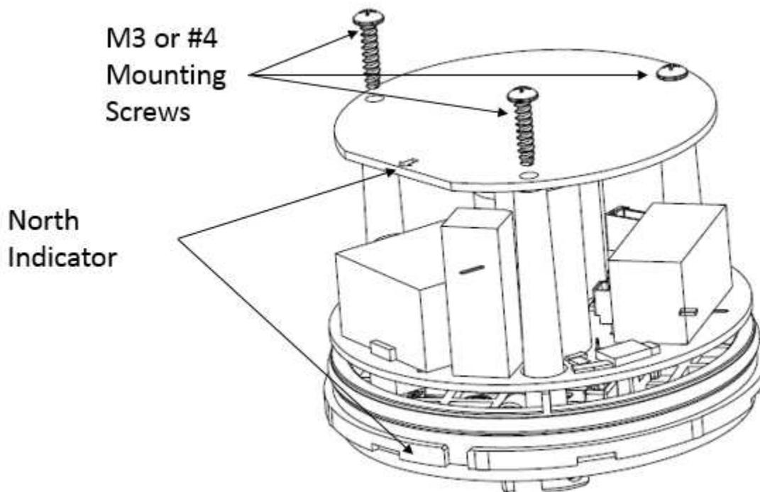
Figure 12. CPCBA mounting
