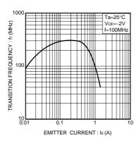
Fig.5 Gain bandwidth product vs. emitter current
