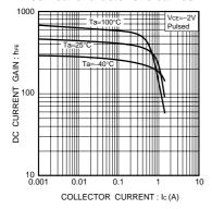
Fig.1 DC current gain vs. collector current
