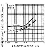
Fig.3 Collector-emitter saturation voltage vs. collector current
