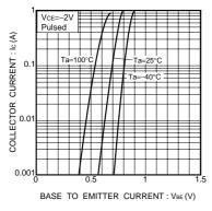
Fig.4 Grounded emitter propagation characteristics
