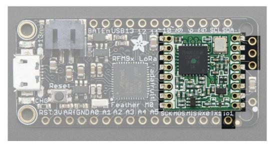
Since not all pins can be brought out to breakouts, due to the small size of the Feather, we use these to control the radio module
