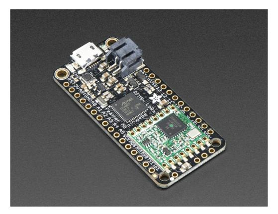
This is the **Adafruit Feather M0 RFM95 LoRa Radio (433 or 900 MHz)**- our take on an microcontroller with a "Long Range (LoRa) (http://adafru.it/mFZ)" packet radio transceiver with built in USB and battery charging. Its an Adafruit Feather M0 with a Long Range radio module cooked in! Great for making wireless networks that are more flexible than Bluetooth LE and without the high power requirements of WiFi. We have other boards in the Feather family, check'em out here (http://adafru.it/17B).
