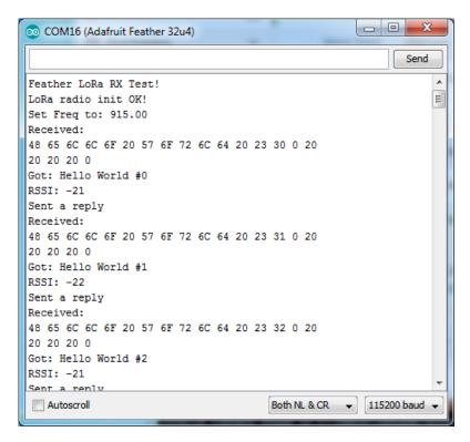
You can see that the library example prints out the hex-bytes received 48 65 6C 6C 6F 20 57 6F 72 6C 64 20 23 30 0 20 20 20 20 0, as well as the ASCII 'string' Hello World. Then it will send a reply.
