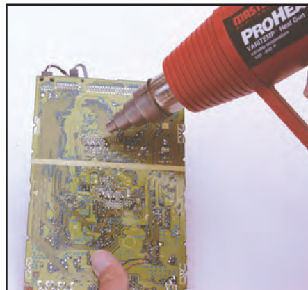
Desolder Circuit Boards
