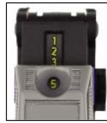
Stepped Stripping Depth For Reduced Friction
