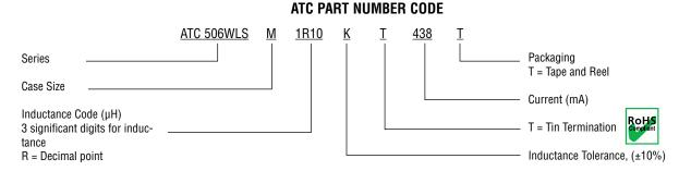
The above part number refers to a 506WLS Series, Case Size M, 1.10 µH inductor, K tolerance (±10%, typ.), with Tin Termination (T), 438 mA, tape and reel packaging.
