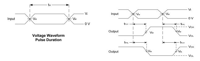
**Voltage Waveform Propagation Delay Times Inverting and Non Inverting Outputs**
