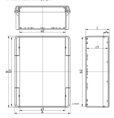
Enclosure B 273126 is closed by 4 corner hinges.
