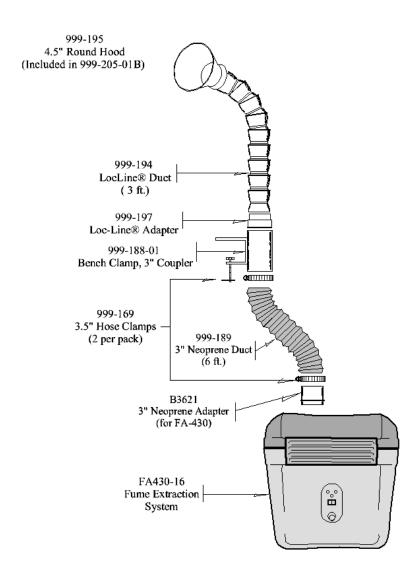
NOTE: Ensure the Neoprene Duct is attached to the longer side of the Neoprene Duct Adapter as measured from the flange.
