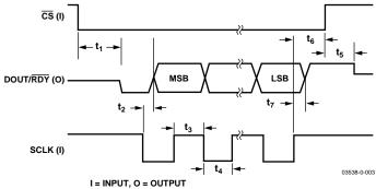
Figure 3. Read Cycle Timing Diagram
