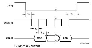
Figure 4. Write Cycle Timing Diagram
