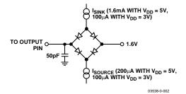
Figure 2. Load Circuit for Timing Characterization
