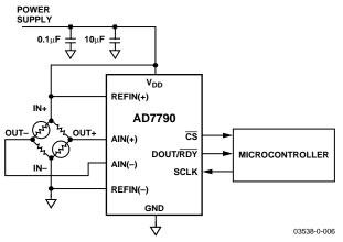
Figure 7. Basic Connection Diagram
