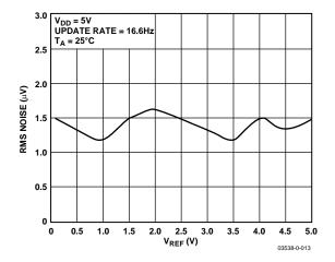
Figure 7. RMS Noise vs. Reference Voltage
