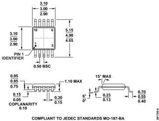
Figure 11. 10-Lead Mini Small Outline Package [MSOP]
