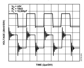
Figure 45. AD8610/AD8620 Driving  $C_L = 10,000 pF$
