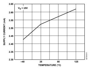
Figure 11. Supply Current vs. Temperature
