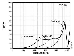
Figure 30. Zout vs. Frequency
