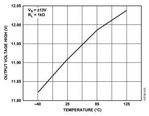
Figure 15. Output Voltage High vs. Temperature
