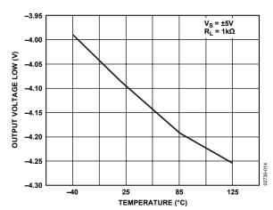
Figure 14. Output Voltage Low vs. Temperature
