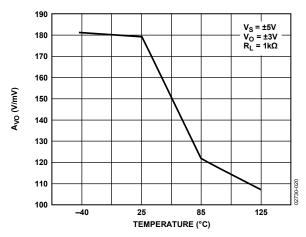
Figure 20. A<sub>VO</sub> vs. Temperature
