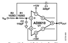
Figure 69. Second-Order, Low-Pass Filter
