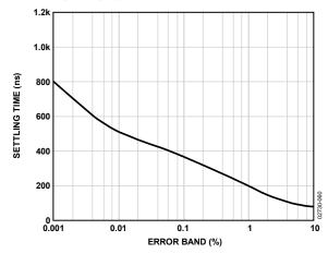
Figure 60. AD8610/AD8620 Settling Time vs. Error Band
