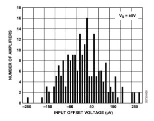
Figure 5. Input Offset Voltage
