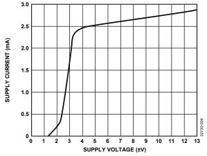
Figure 9. Supply Current vs. Supply Voltage
