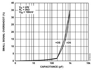
Figure 33. Small Signal Overshoot vs. Load Capacitance
