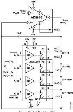
Figure 67. High Precision PGA
