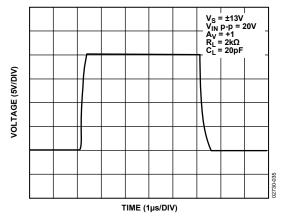
Figure 35. Large Signal Response at G = +1
