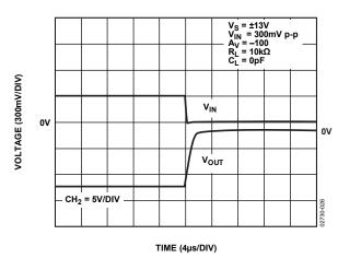
Figure 26. Negative Overvoltage Recovery
