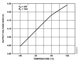
Figure 13. Output Voltage High vs. Temperature
