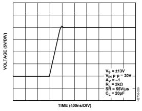
Figure 39. +Slew Rate at G = -1
