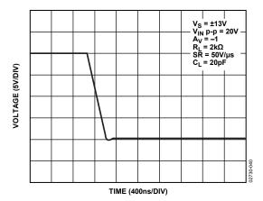
Figure 40. –Slew Rate at G = -1
