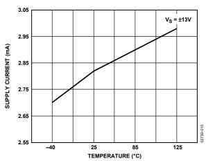
Figure 10. Supply Current vs. Temperature
