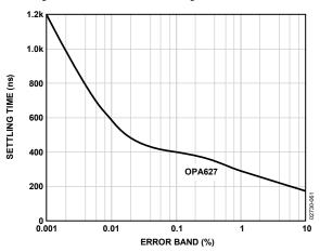
Figure 61. OPA627 Settling Time vs. Error Band
