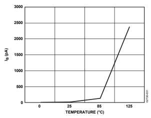
Figure 31. Input Bias Current vs. Temperature
