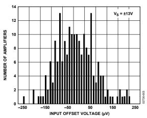
Figure 3. Input Offset Voltage
