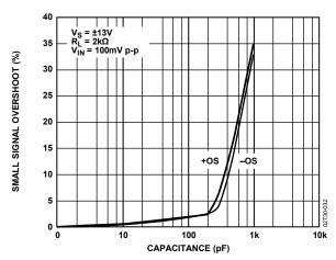
Figure 32. Small Signal Overshoot vs. Load Capacitance
