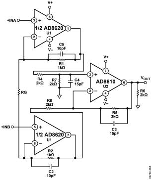
Figure 68. High Speed Instrumentation Amplifier
