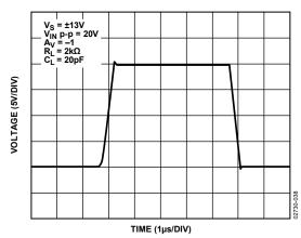
Figure 38. Large Signal Response at G = -1
