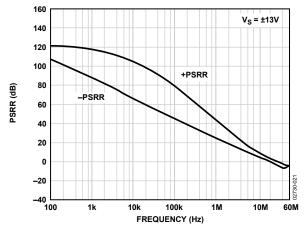
Figure 21. PSRR vs. Frequency
