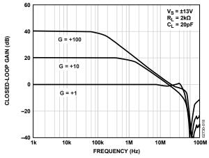
Figure 18. Closed-Loop Gain vs. Frequency
