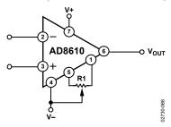
Figure 66. Offset Voltage Nulling Circuit
