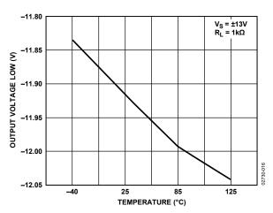
Figure 16. Output Voltage Low vs. Temperature
