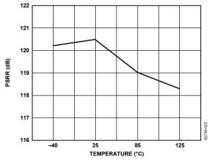
Figure 23. PSRR vs. Temperature
