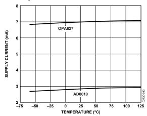
Figure 43. Supply Current vs. Temperature
