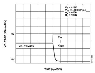
Figure 25. Positive Overvoltage Recovery
