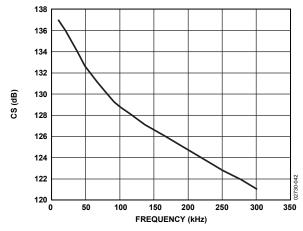
Figure 42. AD8620 Channel Separation Graph
