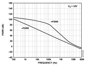
Figure 22. PSRR vs. Frequency
