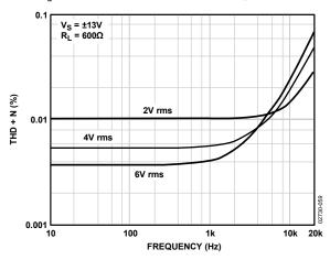
Figure 59. THD + Noise vs. Frequency
