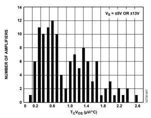
Figure 7. Input Offset Voltage Drift
