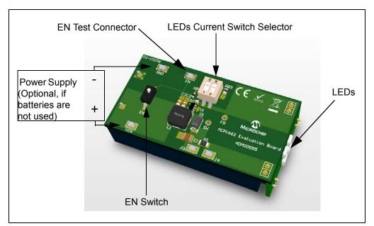
FIGURE 2-2: MCP1662 LED Driver Evaluation Board Setup.
