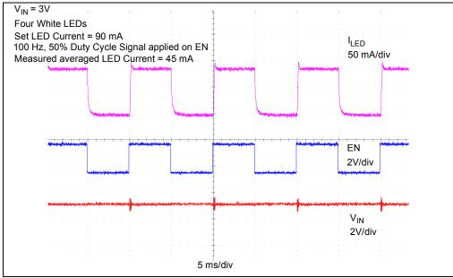
**FIGURE 2-3:** PWM Dimming with MCP1662.
