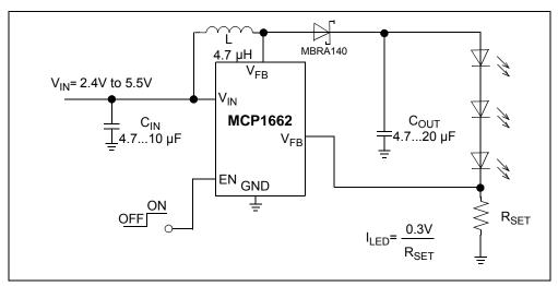
FIGURE 1-1: Typical MCP1662 LED Driver Boost Converter Application.
