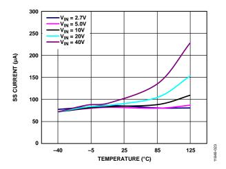
Figure 25. Soft Start (SS) Current vs. Temperature, Multiple Input Voltages ( $V_{\text{N}}$ ),  $V_{\text{OUT}} = 5 \text{ V}$
