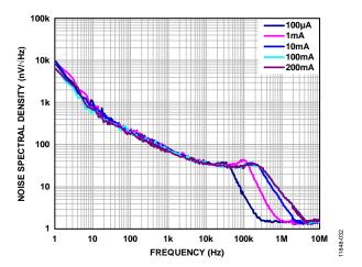
$\textit{Figure 34. Output Noise Spectral Density vs. Frequency, for \textit{Different Loads}}$
