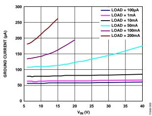
Figure 11. Ground Current vs. Input Voltage (V<sub>IN</sub>)
