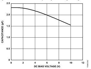
Figure 45. Capacitance vs. Voltage Characteristic
