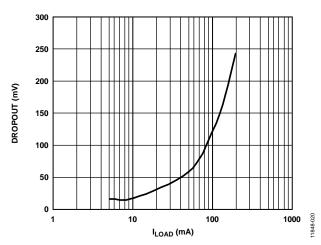
Figure 22. Dropout Voltage vs. Load Current ( $I_{LOAD}$ ),  $V_{OUT} = 3.3 \text{ V}$
