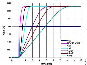
Figure 49. Typical Soft Start Behavior, Different C<sub>SS</sub>
