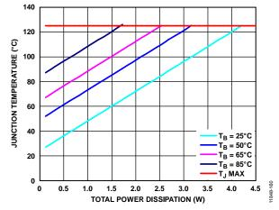
Figure 61. LFCSP Junction Temperature Rise, Different Board Temperatures
