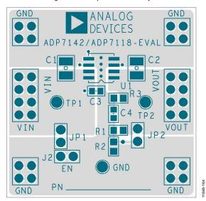
Figure 65. Example SOIC PCB Layout
