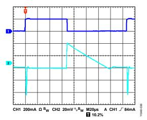
Figure 40. Load Transient Response,  $I_{\rm LOAD}=1$  mA to 200 mA,  $V_{\rm OUT}=1.8$  V,  $V_{\rm IN}=3$  V, CH1 Load Current ( $I_{\rm LOAD}$ ), CH2  $V_{\rm OUT}$
