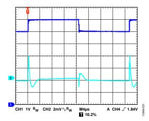
Figure 39. Line Transient Response,  $I_{LOAD}$  = 200 mA,  $V_{OUT}$  = 3.3 V, CH1  $V_{IN}$  CH2  $V_{OUT}$
