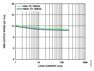
Figure 32. RMS Output Noise vs. Load Current (I<sub>LOAD</sub>)
