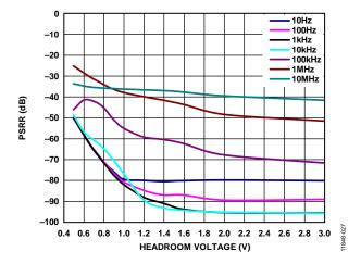
Figure 29. Power Supply Rejection Ratio (PSRR) vs. Headroom Voltage,  $V_{\rm OUT}$  = 3.3 V, for Different Frequencies
