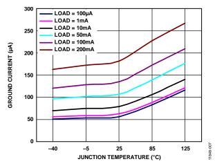
Figure 9. Ground Current vs. Junction Temperature
