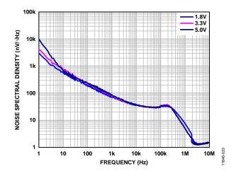
Figure 35. Output Noise Spectral Density vs. Frequency, for Different Output Voltages ( $V_{\rm OUT}$ )
