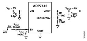
Figure 47. Typical EN Pin Voltage Divider
