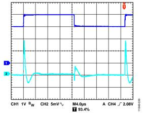
Figure 41. Line Transient Response,  $I_{LOAD}$  = 200 mA,  $V_{OUT}$  = 1.8 V, CH1  $V_{IN}$ , CH2  $V_{OUT}$
