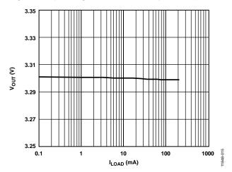
Figure 17. Output Voltage ( $V_{\text{OUT}}$ ) vs. Load Current ( $I_{\text{LOAD}}$ ),  $V_{\text{OUT}}$  = 3.3 V
