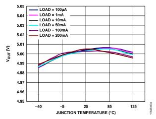
Figure 6. Output Voltage ( $V_{OUT}$ ) vs. Junction Temperature
