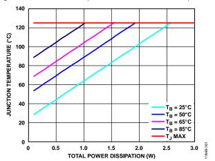
Figure 62. SOIC Junction Temperature Rise, Different Board Temperatures
