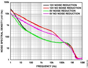
Figure 51. 6 V and 12 V Output Voltage with and Without Noise Reduction
