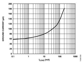
Figure 10. Ground Current vs. Load Current (I<sub>LOAD</sub>)
