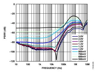
Figure 28. Power Supply Rejection Ratio (PSRR) vs. Frequency,  $V_{\rm OUT}$  = 3.3 V, for Various Headroom Voltages
