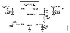
Figure 43. Typical Adjustable Output Voltage Application Schematic
