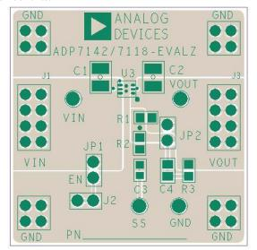
Figure 64. Example LFCSP PCB Layout
