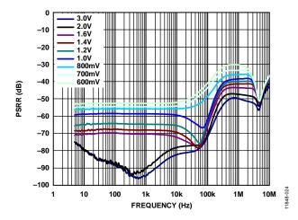
Figure 26. Power Supply Rejection Ratio (PSRR) vs. Frequency,  $V_{\rm OUT}$  = 1.8 V, for Various Headroom Voltages
