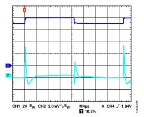
Figure 37. Line Transient Response,  $I_{LOAD}$  = 200 mA,  $V_{OUT}$  = 5 V, CH1  $V_{IN}$ , CH2  $V_{OUT}$
