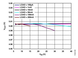
Figure 8. Output Voltage ( $V_{OUT}$ ) vs. Input Voltage ( $V_{IN}$ )
