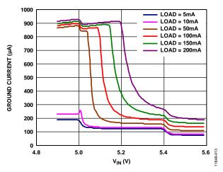
Figure 15. Ground Current vs. Input Voltage ( $V_{IN}$ ) in Dropout,  $V_{OUT} = 5 V$
