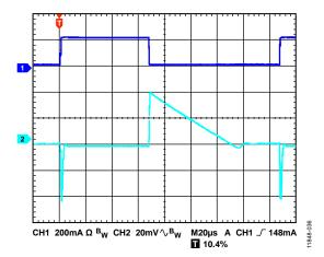
Figure 38. Load Transient Response,  $I_{LOAD} = 1$  mA to 200 mA,  $V_{OUT} = 3.3$  V,  $V_{IN} = 5$  V, CH1 Load Current ( $I_{LOAD}$ ), CH2  $V_{OUT}$
