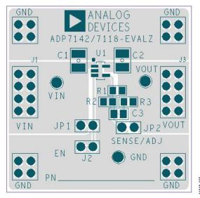
Figure 66. Example TSOT PCB Layout
