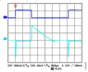
Figure 44. Output Transient Response,  $V_{\rm OUT}$  = 5 V,  $C_{\rm OUT}$  = 2.2  $\mu$ F, CH1 Load Current, CH2  $V_{\rm OUT}$
