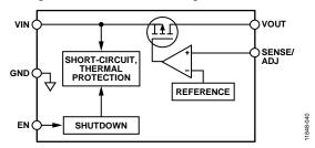
Figure 42. Internal Block Diagram
