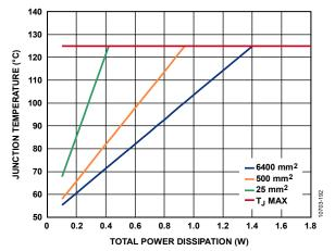
Figure 93. Junction Temperature vs. Total Power Dissipation for the 6-Lead LFCSP,  $T_A = 50^{\circ}C$
