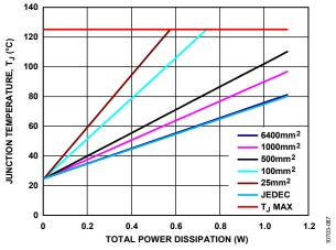
Figure 89. Junction Temperature vs. Total Power Dissipation for the 8-Lead LFCSP,  $T_A = 25^{\circ}C$
