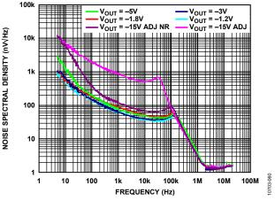
Figure 62. Noise Spectral Density, Various Output Voltages
