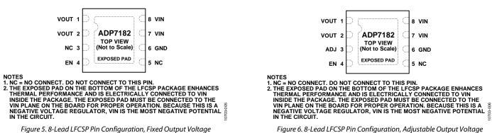
Figure 5. 8-Lead LFCSP Pin Configuration, Fixed Output Voltage
