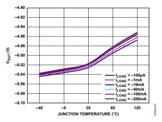
Figure 19. Output Voltage ( $V_{OUT}$ ) vs. Junction Temperature (T<sub>J</sub>),  $V_{OUT} = -5 V$
