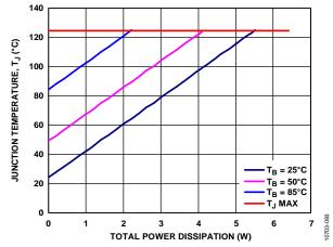
Figure 98. Junction Temperature vs. Total Power Dissipation for the 8-Lead LFCSP,  $T_A = 85^{\circ}$ C
