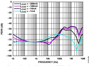
Figure 56. Power Supply Rejection Ratio (PSRR) vs. Frequency,  $V_{OUT} = -3 V$  vs. Different Load Currents ( $I_{LOAD}$ ),  $V_{IN} = -5.5 V$
