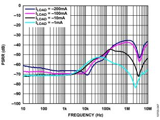
Figure 49. Power Supply Rejection Ratio (PSRR) vs. Frequency,  $V_{OUT} = -1.22$  V vs. Different Load Currents (I<sub>LOAD</sub>),  $V_{IN} = -2.7$  V
