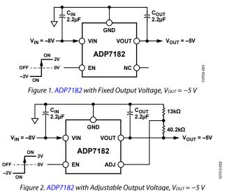
The following fixed output voltages are available from stock: -5 V (3 mm × 3 mm LFCSP), -1.8 V, -2.5 V, -3 V, -5 V (TSOT), -1.2 V, -1.5 V, -2.5 V, -5 V (2 mm × 2 mm LFCSP). Additional voltages are available by special order.
