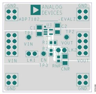
Figure 103. Example of the 5-Lead TSOT PCB Layout
