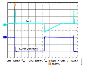
Figure 74. Load Transient Response,  $V_{OUT} = -3$  V,  $I_{LOAD} = -1$  mA to -200 mA, Load Step = 1 A/µs
