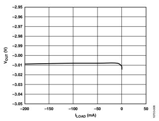
Figure 10. Output Voltage (VOUT) vs. Load Current (ILOAD)
