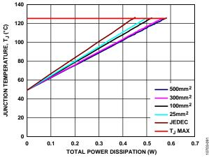
Figure 96. Junction Temperature vs. Total Power Dissipation for the 5-Lead TSOT,  $T_A = 50^{\circ}C$
