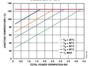
Figure 99. Junction Temperature vs. Total Power Dissipation for the 6-Lead LFCSP,  $T_A = 85^{\circ}C$
