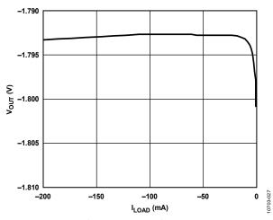
Figure 29. Output Voltage (Vout) vs. Load Current (ILOAD), Vout = -1.8 V
