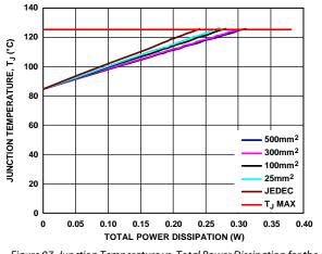
Figure 97. Junction Temperature vs. Total Power Dissipation for the 5-Lead TSOT,  $T_A = 85^{\circ}C$
