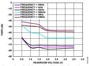
Figure 57. Power Supply Rejection Ratio (PSRR) vs. Headroom Voltage,  $V_{OUT} = -3 V$ , Load Current ( $I_{LOAD}$ ) = -200 mA
