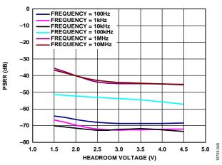
Figure 51. Power Supply Rejection Ratio (PSRR) vs. Headroom Voltage,  $V_{OUT} = -1.22$  V, Load Current ( $I_{LOAD}$ ) = -200 mA
