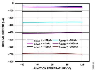
Figure 22. Ground Current vs. Junction Temperature (T<sub>J</sub>),  $V_{OUT} = -5 V$
