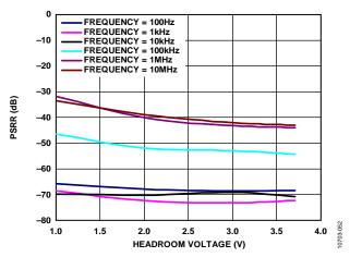
Figure 54. Power Supply Rejection Ratio (PSRR) vs. Headroom Voltage,  $V_{OUT} = -1.8$  V, Load Current ( $I_{LOAD}$ ) = -200 mA
