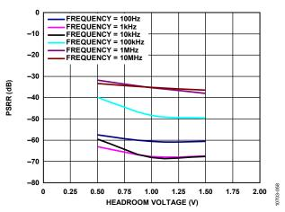
Figure 60. Power Supply Rejection Ratio (PSRR) vs. Headroom Voltage, Adjustable Output Voltage,  $V_{OUT} = -15$  V with Noise Reduction Network, Load Current ( $I_{LOAD}$ ) = -200 mA
