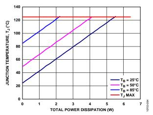
Figure 100. Junction Temperature vs. Total Power Dissipation for the 5-Lead TSOT,  $T_A = 85^{\circ}C$
