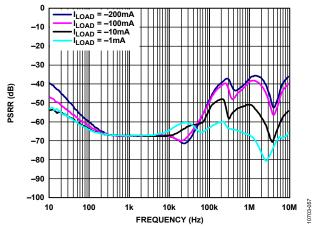
Figure 59. Power Supply Rejection Ratio (PSRR) vs. Frequency, Adjustable Output Voltage,  $V_{OUT} = -15$  V vs. Different Load Currents ( $I_{LOAD}$ ),  $V_{IN} = -16.5$  V with Noise Reduction Network
