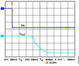
Figure 85. Typical Start-Up Behavior, Negative Going Enable
