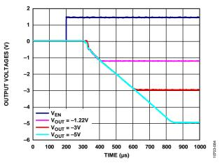
Figure 86. Typical Start-Up Behavior, Different Output Voltages
