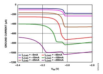
Figure 18. Ground Current vs. Input Voltage (V<sub>IN</sub>) in Dropout
