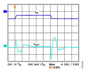
Figure 71. Line Transient Response, 500 mV Step,  $V_{OUT} = -15 V$ , Noise Reduction Network,  $I_{LOAD} = -200 \text{ mA}$
