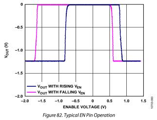
Figure 82 shows the typical hysteresis of the EN pin. This prevents on/off oscillations that can occur due to noise on the EN pin as it passes through the threshold points.
