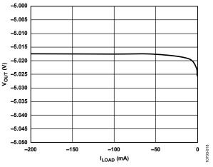
Figure 20. Output Voltage (V<sub>OUT</sub>) vs. Load Current (I<sub>LOAD</sub>),  $V_{OUT} = -5 V$
