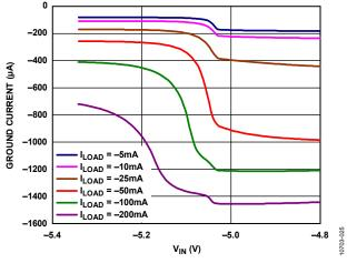
Figure 27. Ground Current vs. Input Voltage ( $V_{IN}$ ) in Dropout,  $V_{OUT} = -5 V$
