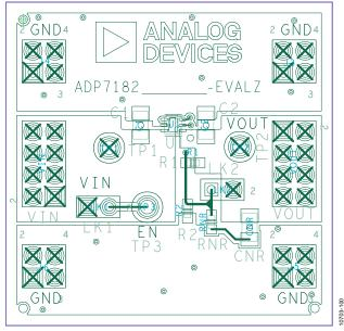
Figure 101. Example of the 6-Lead LFCSP PCB Layout
