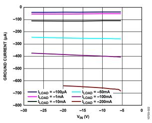
Figure 24. Ground Current vs. Input Voltage ( $V_{IN}$ ),  $V_{OUT} = -5 V$
