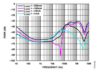
Figure 58. Power Supply Rejection Ratio (PSRR) vs. Frequency, Adjustable Output Voltage,  $V_{OUT} = -15$  V vs. Different Load Currents ( $I_{LOAD}$ ),  $V_{IN} = -15.5$  V with Noise Reduction Network
