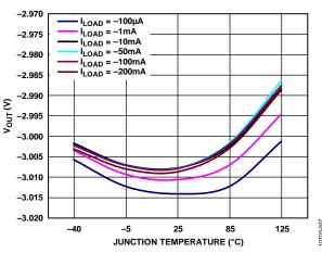
Figure 9. Output Voltage (V<sub>OUT</sub>) vs. Junction Temperature (T<sub>J</sub>)
