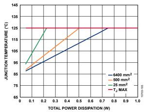
Figure 94. Junction Temperature vs. Total Power Dissipation for the 6-Lead LFCSP,  $T_A = 85^{\circ}C$
