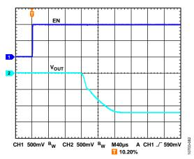
Figure 84. Typical Start-Up Behavior, Positive Going Enable
