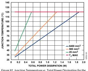
Figure 92. Junction Temperature vs. Total Power Dissipation for the 6-Lead LFCSP,  $T_A = 25^{\circ}C$
