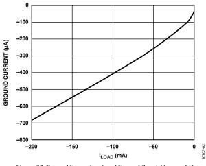
Figure 23. Ground Current vs. Load Current ( $I_{LOAD}$ ),  $V_{OUT} = -5 V$
