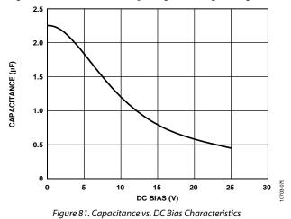
Use Equation 1 to determine the worst-case capacitance accounting for capacitor variation over temperature, component tolerance, and voltage.
