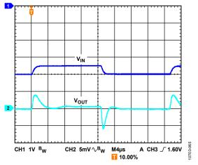
Figure 67. Line Transient Response, 500 mV Step,  $V_{OUT} = -3 V$ ,  $I_{LOAD} = -200 \text{ mA}$
