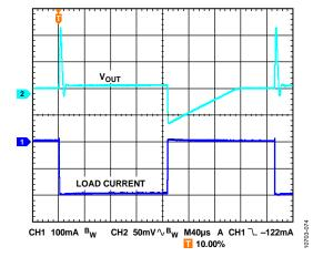
Figure 76. Load Transient Response,  $V_{OUT} = -15$  V,  $I_{LOAD} = -1$  mA to -200 mA, Load Step = 1 A/µs, Noise Reduction Network
