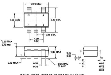
\*COMPLIANT TO JEDEC STANDARDS MO-193-AB WITH THE EXCEPTION OF PACKAGE HEIGHT AND THICKNESS.
