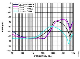
Figure 55. Power Supply Rejection Ratio (PSRR) vs. Frequency,  $V_{OUT} = -3$  V vs. Different Load Currents (I<sub>LOAD</sub>),  $V_{IN} = -4.0$  V
