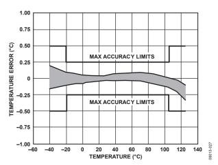
Figure 4. Temperature Accuracy at 3 V
