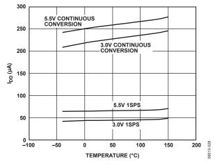
Figure 6. Operating Supply Current vs. Temperature
