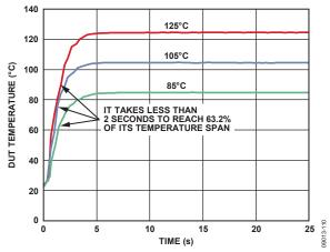
Figure 10. Thermal Response Time
