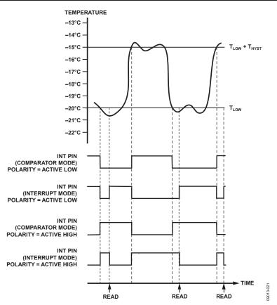
$\textit{Figure 19. INT Output Temperature Response Diagram for $T_{LOW}$ Under temperature Events}$
