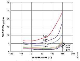
Figure 7. Shutdown Current vs. Temperature
