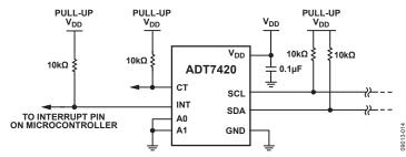
Figure 13. Typical I<sup>2</sup>C Interface Connection
