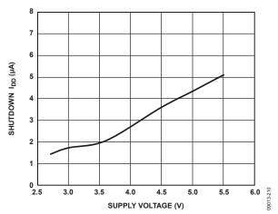
Figure 9. Shutdown Current vs. Supply Voltage
