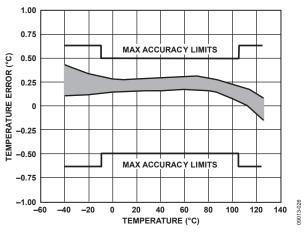
Figure 5. Temperature Accuracy at 5 V
