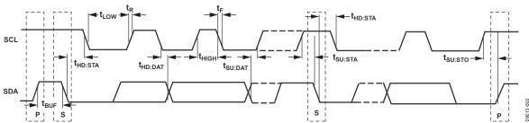
Figure 2. Serial Interface Timing Diagram
