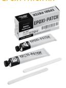
Applications include sealing rivets, bolts, metal joints, seams and welds, cement cracks, pipe couplings, joints and tees. Each kit has two tubes of material, application instructions and a mixing stick. When the resin and hardener are mixed, a gray epoxy is formed which cures at room temperature, has high adhesion and will not sag. It is resistant to oils, acids and chemicals.
