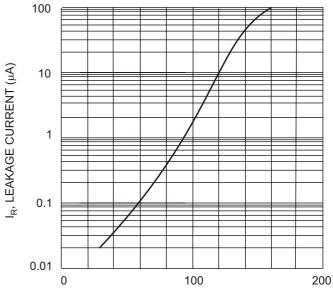
$\label{eq:total_total_total} \textbf{T}_{j}, \, \text{JUNCTION TEMPERATURE (°C)}$  Fig. 2 Leakage Current vs Junction Temperature
