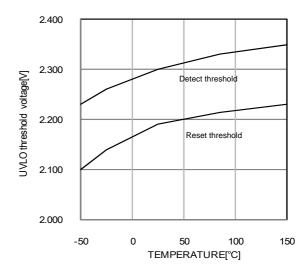
Fig.7 UVLO detect threshold Vs temp
