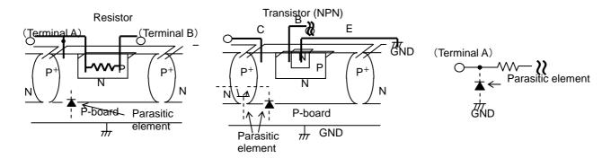
Fig.36 Simplified structure of a Bipolar IC
