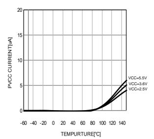
Fig.16 VCC input current vs Temp (STB OFF)
