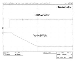
Fig.29 CH1 Soft start waveform
