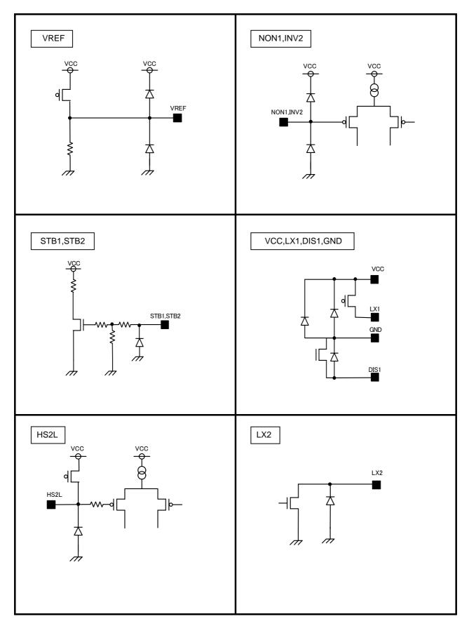
Fig.35 I/O Equivalence Circuit
