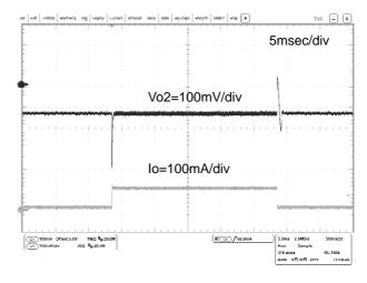
Fig.28 CH2 Output current response (output current : 10mA ⇔ 100mA)
