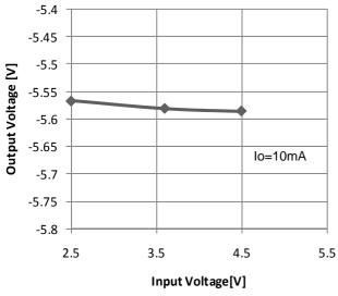
Fig.25 CH1 Output voltage vs Input voltage
