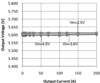
Fig.24 CH2 Output voltage vs Output Current
