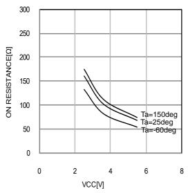
Fig.14 NON1 discharge SW ON registance vs VCC
