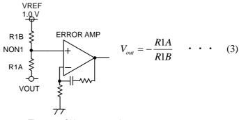
Fig.33 CH1output setting
