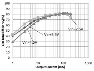
Fig.21 CH1 Power conversion efficiency vs output current
