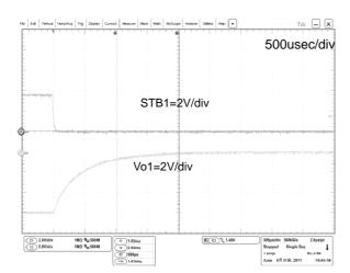
Fig.31 CH1 Discharge waveform [500usec/div] (STB1:High  $\rightarrow$  Low)
