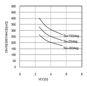
Fig.12 HS2L high side FET ON registance vs VCC
