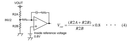
Fig.34 CH2 output setting
