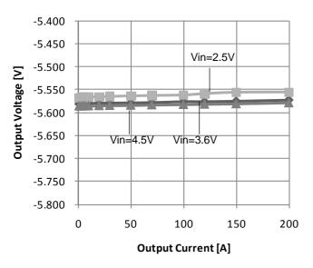
Fig.23 CH1 Output voltage vs Output Current
