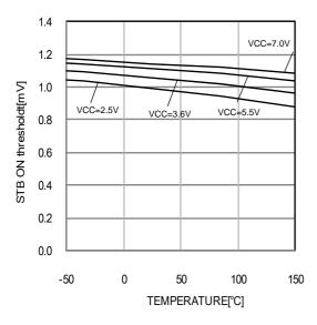
Fig.8 STB ON threshold voltage vs temp
