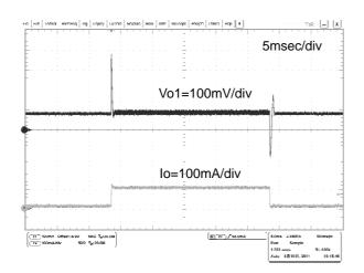
Fig.27 CH1 Output current response (output current : 10mA ⇔ 100mA)
