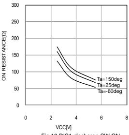
Fig.13 DIS1 discharge SW ON registance vs VCC
