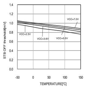
Fig.9 STB OFF threshold voltage vs temp
