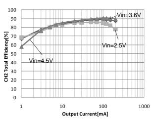
Fig.22 CH2 Power conversion efficiency vs output current
