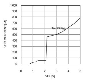
Fig.15 VCC input current vs VCC (STB ON)
