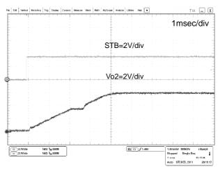
Fig.30 CH2 Soft start waveform
