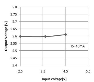
Fig.26 CH2 Output voltage vs Input voltage
