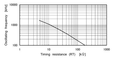
Fig.8 Oscillating frequency - Timing resistance (RRT)
