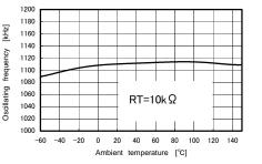
Fig.4 Oscillating frequency – Ambient temperature  $(RT=10k \Omega)$
