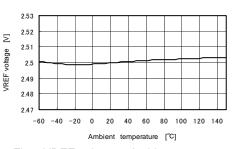
VREF voltage vs. Ambient temperature
