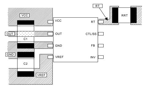
C1 : Capacitor terminals have to be close enough to terminals of VCC and GND. It is safe to pass OUT signal line under C1.
