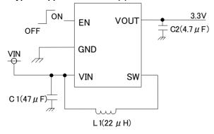
Figure 1. Application Circuit
