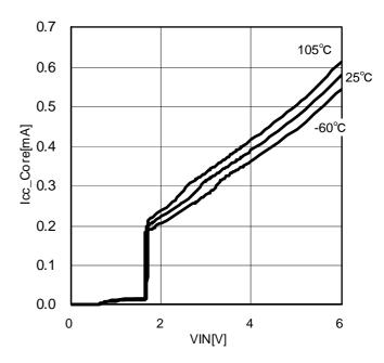
Figure 6. Core Current (This is only VIN current. Not include SW current)
