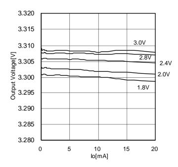
Figure 11. Load-Regulation[Ta=-30°C]
