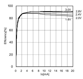
Figure 8. Efficiency[Ta=-30°C]
