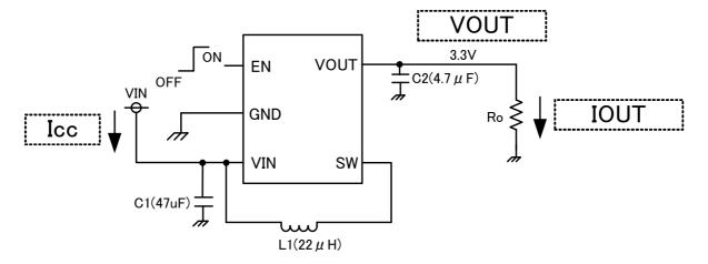
Figure 17. Measure circuit
