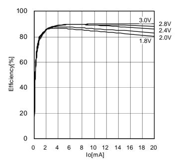
Figure 10. Efficiency[Ta=-85°C]
