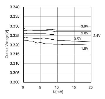
Figure 13. Load-Regulation[Ta=-85°C]
