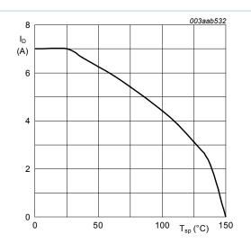
Fig. 2. Continuous drain current as a function of solder point temperature
