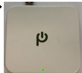
Figure 3. PowerByProxi ProxiPoint Transmitter
