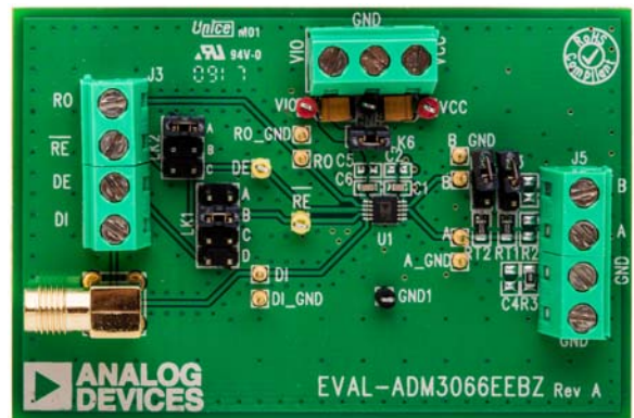
Figure 1. EVAL-ADM3066EEBZ Evaluation Board
