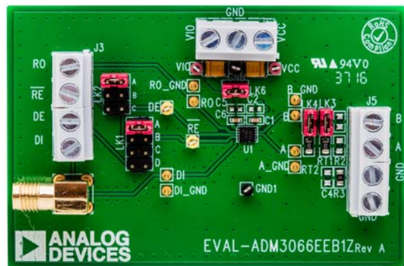
Figure 2. EVAL-ADM3066EEB1Z Evaluation Board
