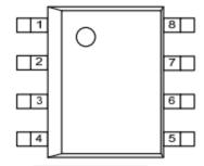
Figure 2. Pin Assignment (Top View)
