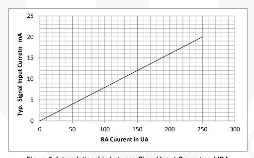
Figure 6: Interrelationship between Signal Input Current and IRA
