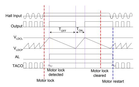
FAN8412M/FAN8413M features a lock detection and an automatic restart. The functions can be operated as follows. When the rotor is locked, there is no change in input signal of hall amplifier.
