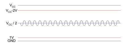
It is recommended that R1 and R3 should have the same value to make the output signal of hall sensor centered as V<sub>CC</sub>/2.
