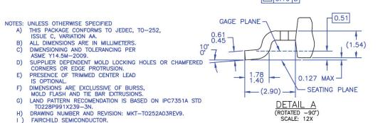
Figure 19. TO252 (D-PAK), Molded, 3-Lead, Option AA&AB
