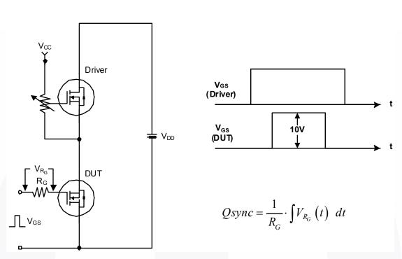
Figure 18. Total Gate Charge Qsync. Test Circuit & Waveforms
