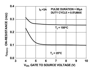
Figure 4. On-Resistance vs Gate to Source Voltage
