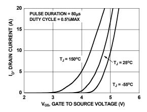
Figure 5. Transfer Characteristics
