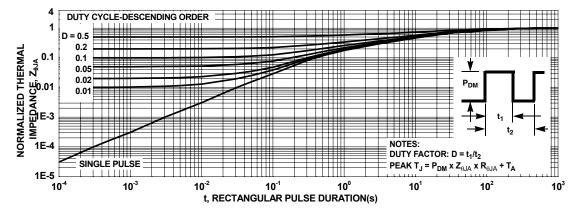
Figure 13. Transient Thermal Response Curve
