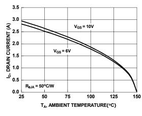
Figure 10. Maximum Continuous Drain Current vs
