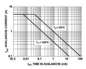
Figure 9. Unclamped Inductive Switching Capability
