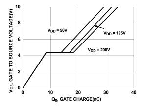
Figure 7. Gate Charge Characteristics
