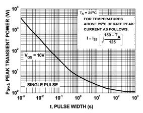
Figure 12. Single Pulse Maximum Power Dissipation
