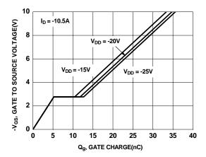
Figure 7. Gate Charge Characteristics
