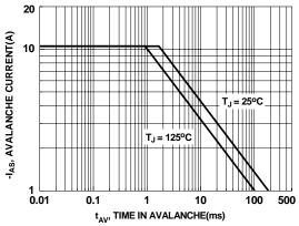
Figure 9. Unclamped Inductive Switching Capability
