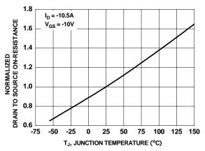
Figure 3. Normalized On-Resistance vs Junction Temperature
