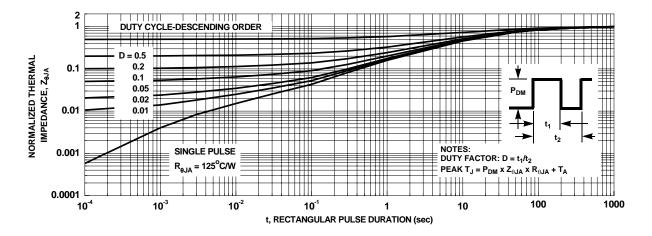
Figure 13. Transient Thermal Response Curve
