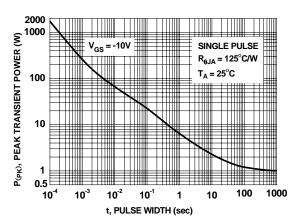
Figure 12. Single Pulse Maximum Power Dissipation
