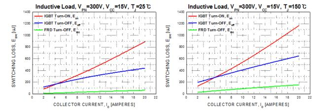
Figure 6. Switching Loss Characteristics
