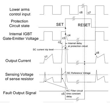
Figure 12. Short-Circuit Current Protection (Low-Side Operation only)
