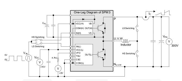
Figure 5. Example Circuit for Switching Test
