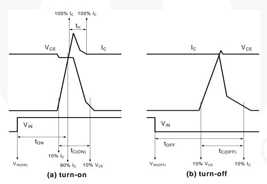
Figure 4. Switching Time Definition
