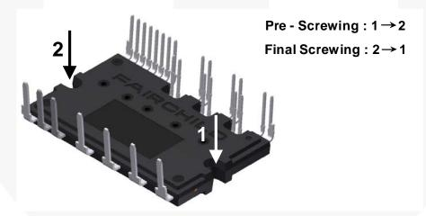
Figure 9. Mounting Screws Torque Order
