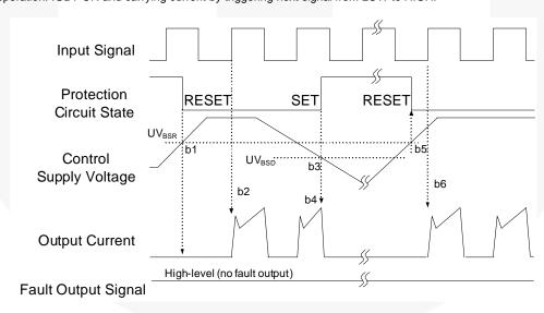
Figure 11. Under-Voltage Protection (High-Side)
