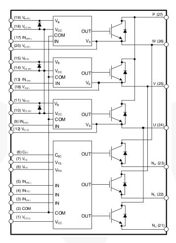
Figure 3. Internal Block Diagram
