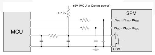
Figure 13. Recommended CPU I/O Interface Circuit
