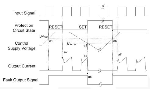
Figure 10. Under-Voltage Protection (Low-Side)
