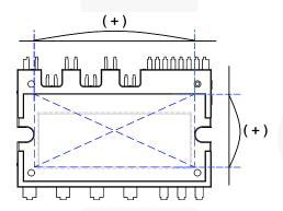
Figure 8. Flatness Measurement Position
