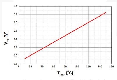
Figure 7. Temperature Profile of V<sub>TS</sub> (Typical)
