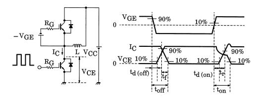
Switching loss measurement waveforms
