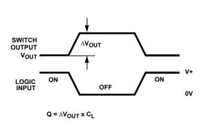
FIGURE 2A. MEASUREMENT POINTS
