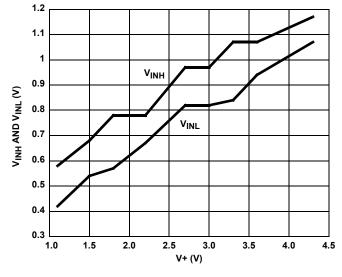
FIGURE 13. DIGITAL SWITCHING POINT vs SUPPLY VOLTAGE
