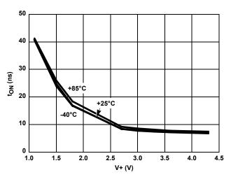
FIGURE 11. TURN - ON TIME vs SUPPLY VOLTAGE
