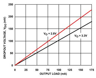
FIGURE 7. DROPOUT VOLTAGE vs LOAD CURRENT
