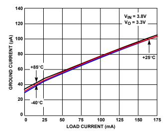
FIGURE 10. GROUND CURRENT vs LOAD
