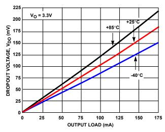
FIGURE 8. DROPOUT VOLTAGE vs LOAD CURRENT
