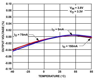
FIGURE 4. OUTPUT VOLTAGE vs TEMPERATURE
