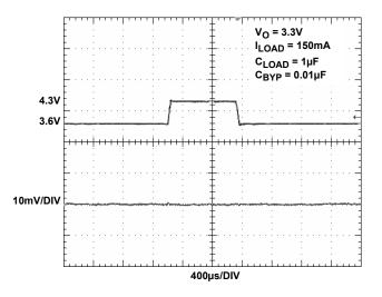
FIGURE 13. LINE TRANSIENT RESPONSE, 3.3V OUTPUT
