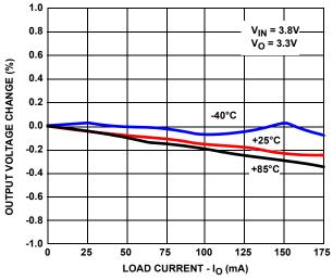
FIGURE 3. OUTPUT VOLTAGE vs LOAD CURRENT
