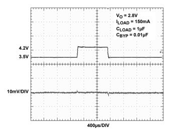
FIGURE 14. LINE TRANSIENT RESPONSE, 2.8V OUTPUT
