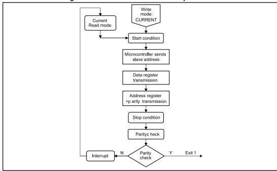
Figure 25: Current write mode flow chart procedure
