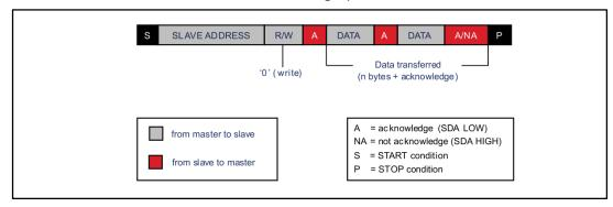
Figure 6: A master reads data from the slave immediately after the first byte
