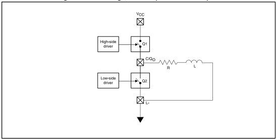
When a power stage output (C/Q or L+) is connected to an inductance, the energy stored in the load is:
