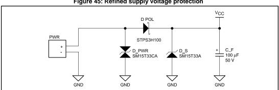
Figure 45: Refined supply voltage protection
