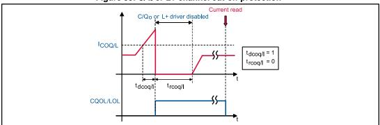
Figure 39: C/Q or L+ channel current limitation and cut-off protection with latched restart
