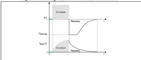
Figure 21: Fast demagnetization waveform. Load connected to L-
