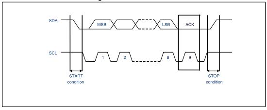
Figure 8: I<sup>2</sup>C communication
