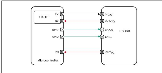
Figure 36: Block diagram communication mode
