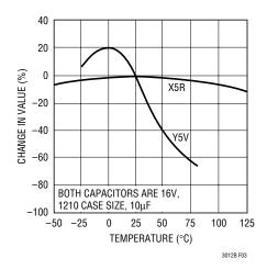
Figure 3. Ceramic Capacitor Temperature Characterics
