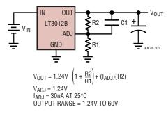
Figure 1. Adjustable Operation
