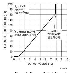
Figure 4. Reverse Output Current
