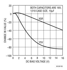
Figure 2. Ceramic Capacitor DC Bias Characterics
