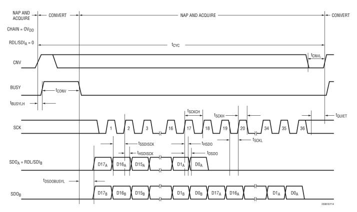
Figure 14. Chain Mode Timing Diagram
