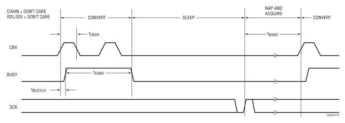
Figure 15. Sleep Mode Timing Diagram
