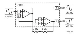
Figure 5a. LT1469 Converting a ±10.24V Single-Ended Signal to a ±20.48V Differential Input Signal
