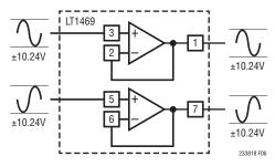
Figure 6. LT1469 Buffering a Fully Differential Signal Source
