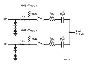
Figure 3. The Equivalent Circuit for the Differential Analog Input of the LTC2338-18
