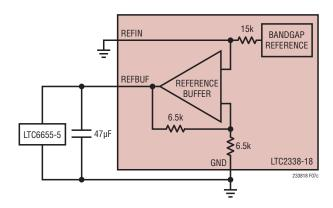
Figure 7c. Overdriving REFBUF Using the LTC6655-5
