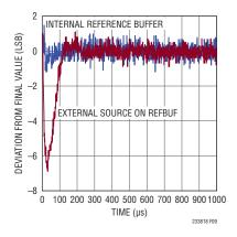
Figure 9. Transient Response of the LTC2338-18
