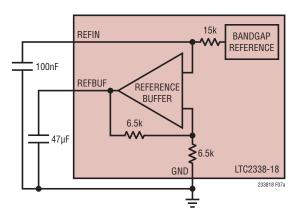
Figure 7a.LTC2338-18 Internal Reference Circuit
