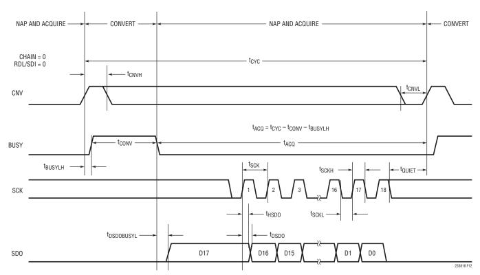
Figure 12. Using a Single LTC2338-18 in Normal Mode
