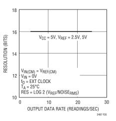
Figure 35. Resolution (Noise\_{RMS}  $\leq$  1LSB) vs Output Data Rate and Temperature
