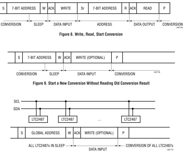
Figure 10. Synchronize Multiple LTC2487s with a Global Address Call
