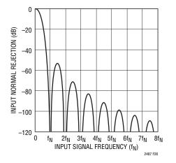
Figure 26. Input Normal Mode Rejection 2x Speed Mode
