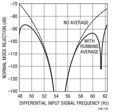
Figure 28. Input Normal Mode Rejection 2x Speed Mode with and Without Running Averaging
