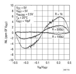
Figure 16. INL vs Differential Input Voltage and Reference Source Resistance for  $C_{REF} > 1\mu F$
