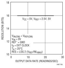
Figure 36. Resolution (INL<sub>MAX</sub>  $\leq$  1LSB) vs Output Data Rate and Temperature 2487ff
