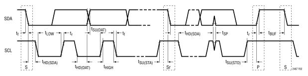
Figure 2. Definition of Timing for Fast/Standard Mode Devices on the  $I^2C$  Bus
