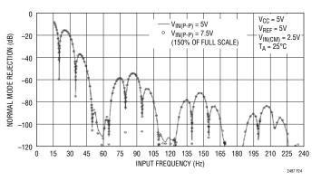
Figure 24. Measure Input Normal Mode Rejection vs Input Frequency with Input Perturbation of 150% (60Hz Notch)
