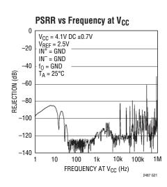
PSRR vs Frequency at  $V_{CC}$
