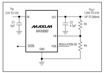
Figure 3. Adjustable Output Using External Feedback Resistors
