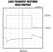
$$\begin{split} &C_{H1} = I_{OUT},\, 12.5 \text{mA/div} \\ &C_{H2} = V_{OUT},\, 100 \text{mV/div},\, \text{AC COUPLED} \\ &V_{IN} = 5.2 \text{V},\, V_{OUT(NOMINAL)} = 5 \text{V} \end{split}$$
