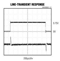
$\begin{array}{l} C_{H1} = V_{IN}, 500mV/div, AC~COUPLED\\ C_{H2} = V_{OUT}, 20mV/div, AC~COUPLED\\ V_{OUT} = 5V, I_{OUT} = 5mA \end{array}$
