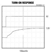
$\begin{aligned} &C_{H1} = \overline{SHDN}, \, 2V/div \\ &C_{H2} = V_{OUT}, \, 1V/div \\ &V_{IN} = 4.0V \end{aligned}$
