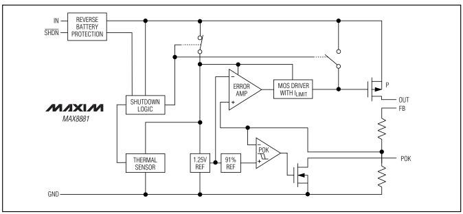
Figure 2. Functional Diagram
