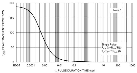
Figure 5. Single Pulse Maximum Power Dissipation
