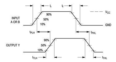
Figure 1. Switching Waveforms
