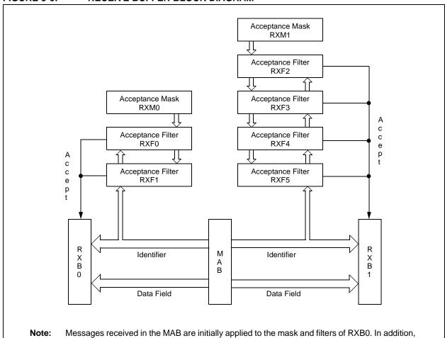
Messages received in the MAB are initially applied to the mask and filters of RXB0. In addition, only one filter match occurs (e.g., if the message matches both RXF0 and RXF2, the match will be for RXF0 and the message will be moved into RXB0).
