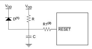
Note 1: The diode, D, helps discharge the capacitor quickly when  $V_{\mbox{\scriptsize DD}}$  powers down.
