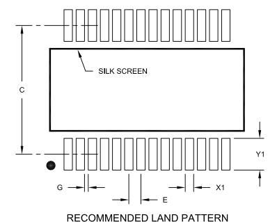
MILLIMETERS Units **Dimension Limits** MIN NOM MAX Contact Pitch Ε 0.65 BSC Contact Pad Spacing С 7.20 Contact Pad Width (X28) X1 0.45 Contact Pad Length (X28) Y1 1.75 Distance Between Pads G 0.20
