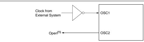
Note 1: A resistor to ground may be used to reduce system noise. This may increase system current.
