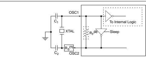
Note 1: A Series Resistor (R<sub>S</sub>) may be required for AT strip-cut crystals.
