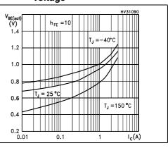
Figure 8. Base-emitter on voltage
