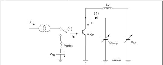
Figure 12. Inductive load switching test circuit
