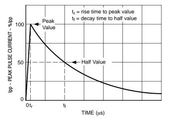
Figure 5. Exponential Decay Pulse Waveform
