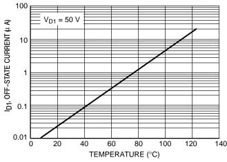
Figure 1. Off–State Current versus Temperature
