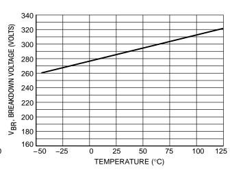
Figure 2. Breakdown Voltage versus Temperature
