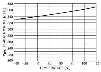
Figure 3. Breakover Voltage versus Temperature
