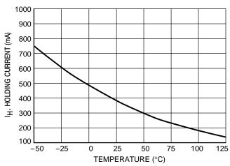
Figure 4. Holding Current versus Temperature
