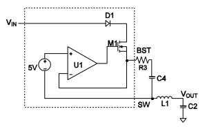
Figure 5: Internal Bootstrap Charging Circuit
