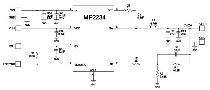
Figure 9: 12V<sub>IN</sub>, 5V/2A Output
