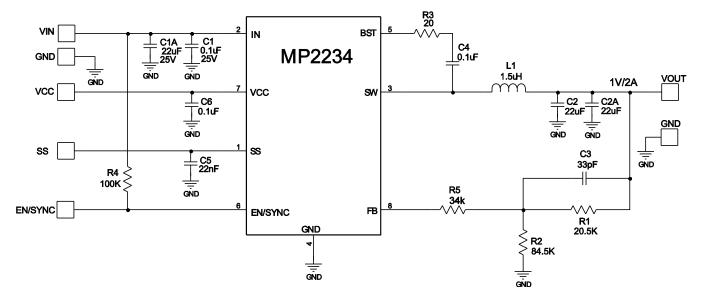
Figure 14: 12V<sub>IN</sub>, 1V/2A Output
