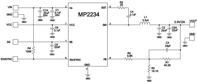
Figure 11: 12V<sub>IN</sub>, 2.5V/2A Output
