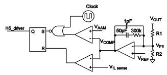
Figure 4: Simplified AAM Control Logic
