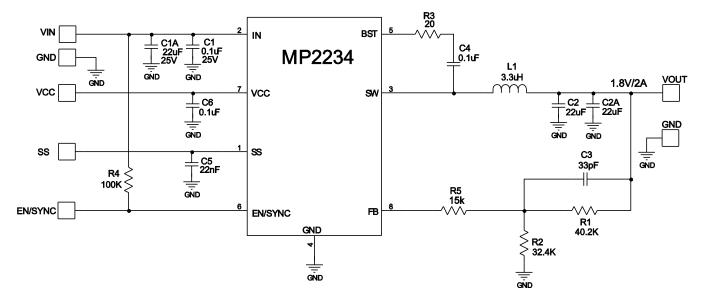
Figure 12: 12V<sub>IN</sub>, 1.8V/2A Output
