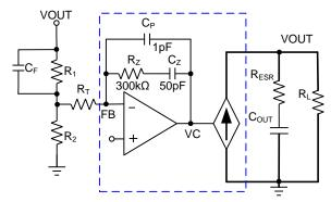
Figure 6: Equivalent Control Loop Model
