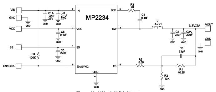
Figure 10: 12V<sub>IN</sub>, 3.3V/2A Output
