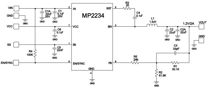
Figure 13: 12V<sub>IN</sub>, 1.2V/2A Output
