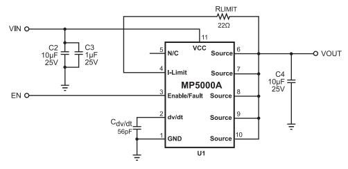
Figure 4—Typical Application Schematic
