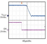
**Short Circuit Current Device Enabled Into Short**
