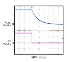
Turn On Delay and Rise Time With 10µF Load
