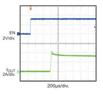
**Short Circuit Current Device Enabled Into Short and Thermal Shut Down (EN Floating)** C<sub>dv/dt</sub>=0
